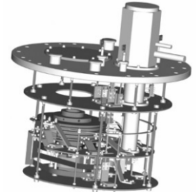
Ansaldo Breda CRIS 1 Tesla cryogenic-free solenoid magnet
