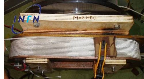
INFN-Genova 2.35 Tesla dipole magnet for particle physics
