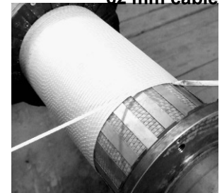
CERN MgB2 cable with I_c > 17 kA, 6 mm in diameter Scaled up to 125 kA on a 62 mm cable
